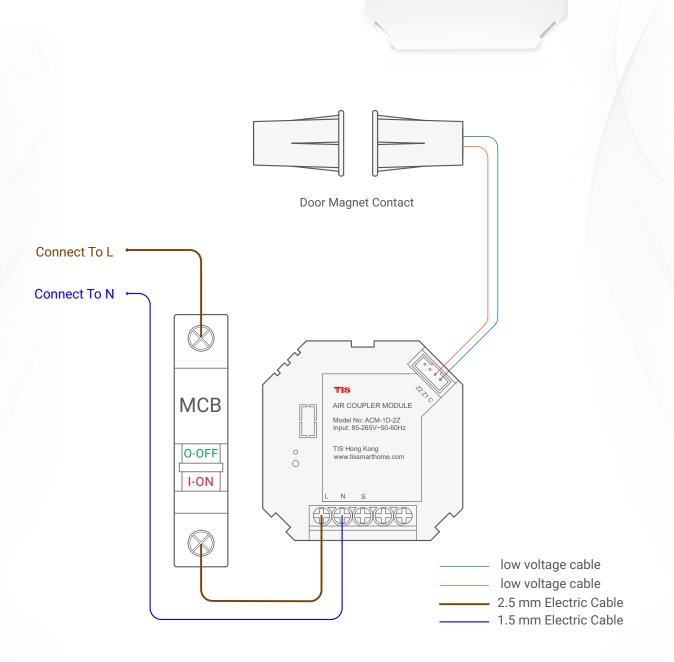
Figure 3: ACM-1D-2Z & Magnetic Door Contact Connection Diagram
