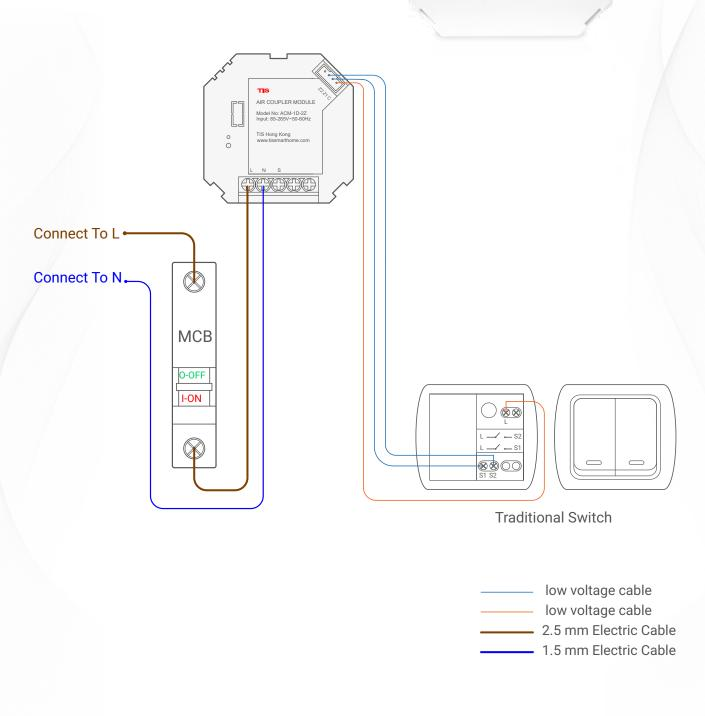
Figure 4: ACM-1D-2Z & Traditional Switch Connection Diagram
