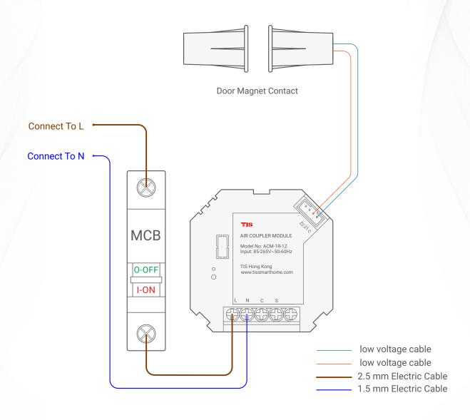
▲ Figure 4: ACM-1R-1Z & Magnetic Door Contact Connection Diagram
