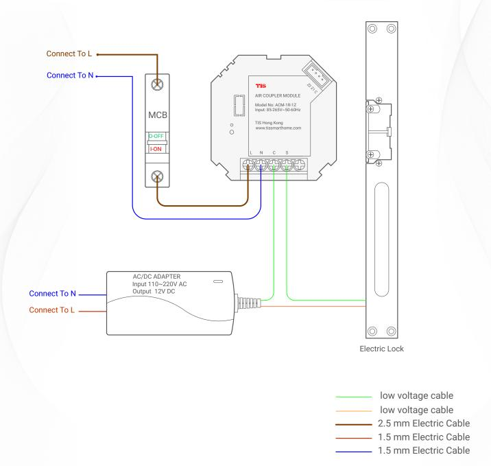
Figure 2: ACM-1R-1Z & Electric Lock Connection Diagram
