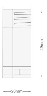
Figure 6: Module's Dimensions
