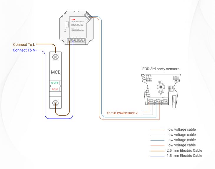
Figure 3: ACM-1R-1Z & 3<sup>rd</sup> Party Sensor Connection Diagram
