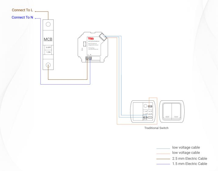
▲ Figure 3: ACM-3Z-IN & Traditional Switch Connection Diagram
