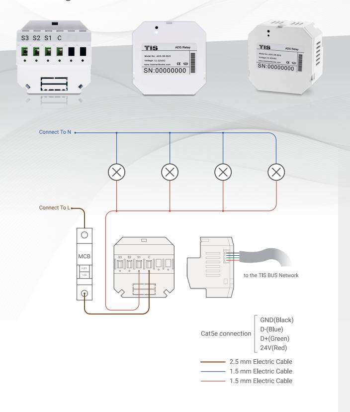
Figure 1: ADS-3R-BUS & Lights Connection Diagram
