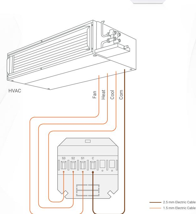
Figure 3: ADS-3R-BUS & HVAC6-3-A-T Connection Diagram
