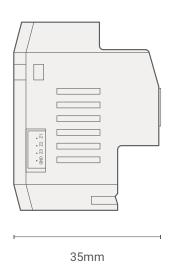
Figure 5: Module's Dimensions
