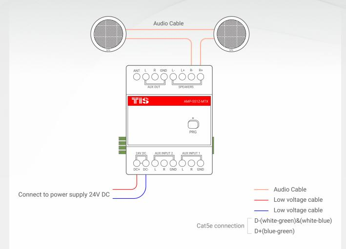
Figure 1: Ceiling-Mount Speaker Connection Diagram (Series Circuit)
