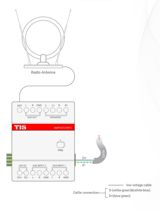
Figure 6: Radio Antenna Connection Diagram
