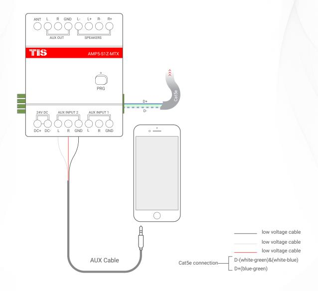
Figure 5: AUX Cable Connection Diagram
