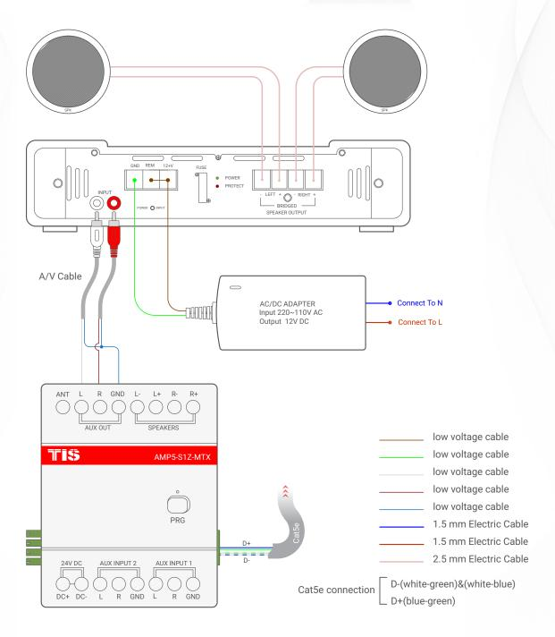
Figure 3: AMP-5S1Z-MTX & Amplifier Connection Diagram
