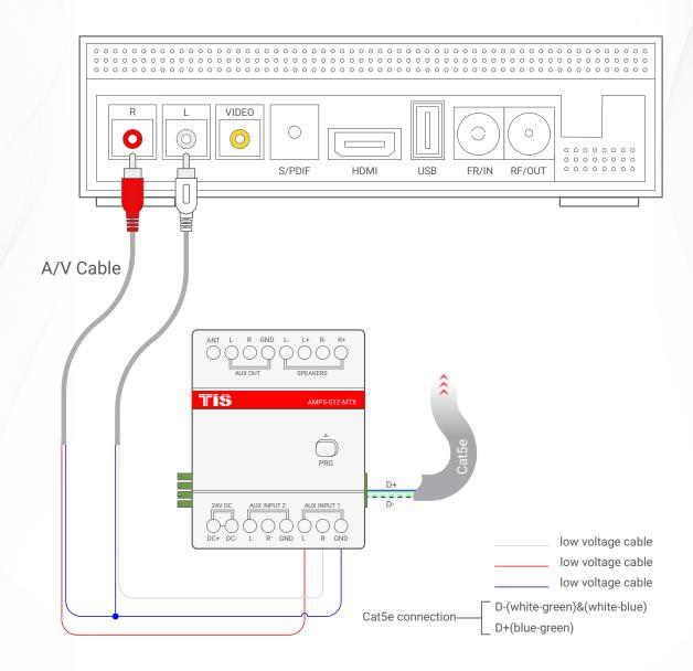
Figure 4: AMP-5S1Z-MTX & A/V Receiver Connection Diagram
