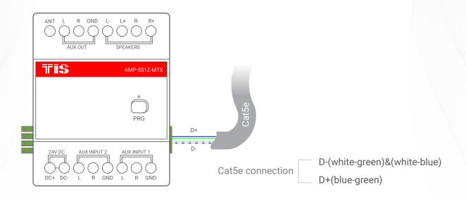
Figure 9: Bus Connection Color Coding
