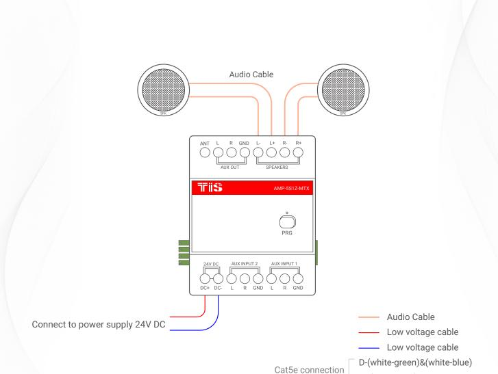
▲ Figure 2: Ceiling-Mount Speaker Connection Diagram (Parallel Circuit)
