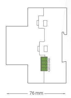
Figure 10: Module Dimensions
