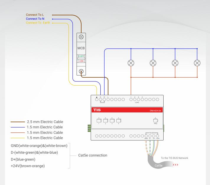
Figure 1: Lights Connection Diagram
