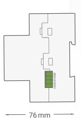
Figure 4: Module Dimensions
