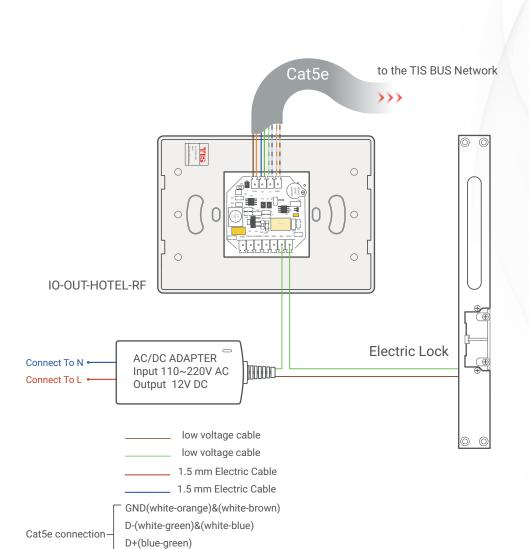
Figure 2: IO-OUT-HOTEL-RF & Electric Lock Connection Diagram
