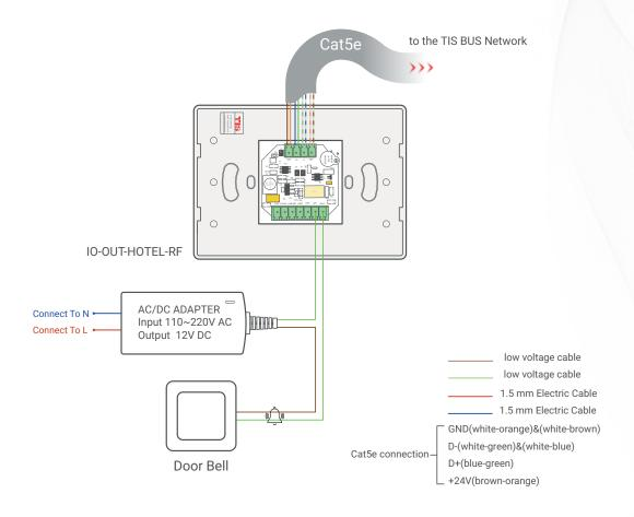
▲ Figure 3: IO-OUT-HOTEL-RF & Door Bell Unit Connection Diagram
