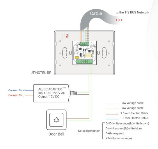
▲ Figure 2: IO-OUT-HOTEL & Door Bell Unit Connection Diagram
