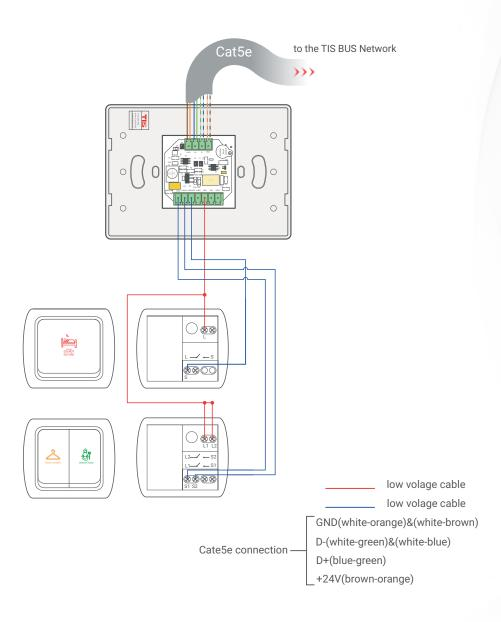
▲ Figure 3: IO-OUT-HOTEL & Traditional Light Switch Connection Diagram
