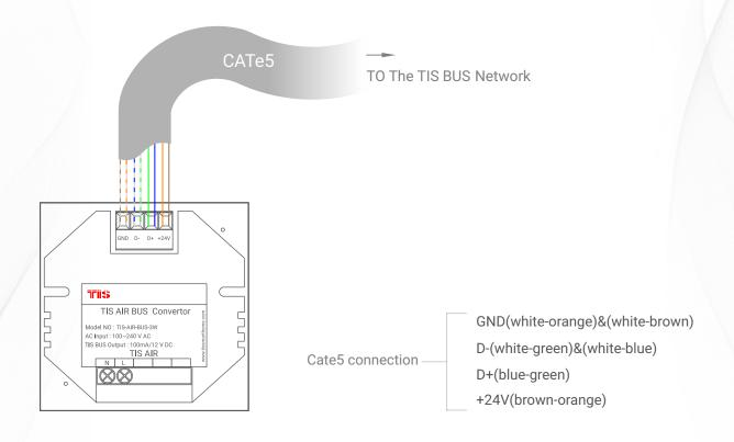
Figure 2: AIR-BUS-3W Bus Connection Diagram
