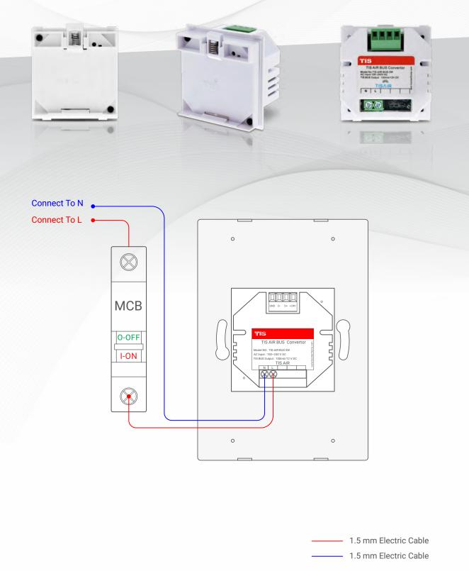
Figure 1: AIR-BUS-3W Configuration Diagram
