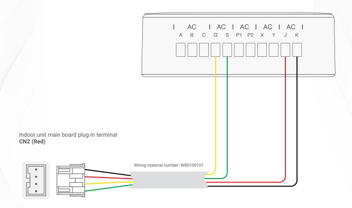
▲ TIS Ducted AC Gateway & Hitachi US Air Duct Wiring Guide
