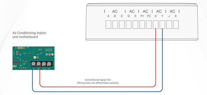
▲ TIS Ducted AC Gateway & Panasonic Multi-Connection Wiring Guide
