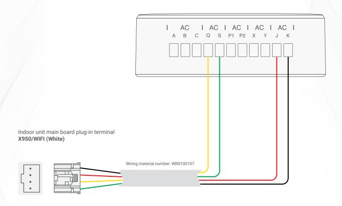
▲ TIS Ducted AC Gateway & Hisense N+ Air Duct Wiring Guide
