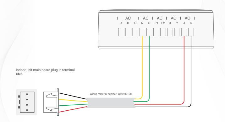
▲ TIS Ducted AC Gateway & Gree Four-Core Wiring Guide
