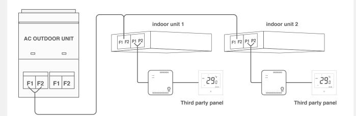
TIS Ducted AC Gateway & AC Outdoor Unit Wiring Guide
