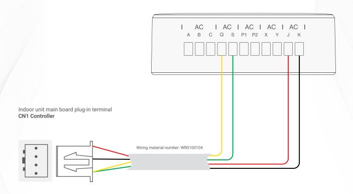
▲ TIS Ducted AC Gateway & Haier Air Duct Wiring Guide
