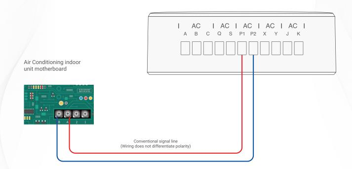
▲ TIS Ducted AC Gateway & Hisense Multi-Connection Wiring Guide
