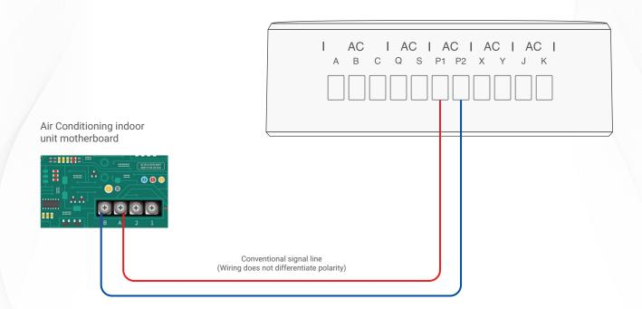
▲ TIS Ducted AC Gateway & Hitachi Multi-Line Connection Guide
