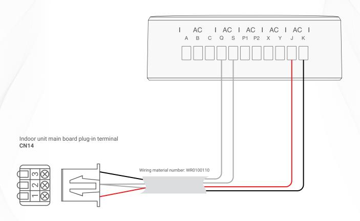
▲ TIS Ducted AC Gateway & Fujitsu Wiring Guide
