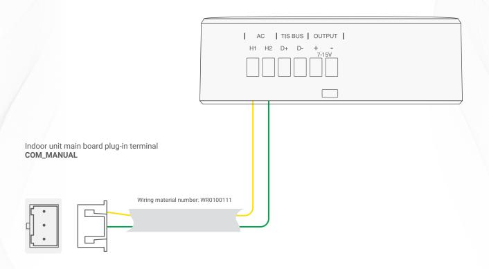
▲ TIS Ducted AC Gateway & Gree Two-Core Wiring Guide
