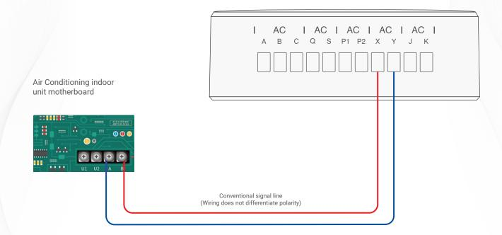
▲ TIS Ducted AC Gateway & Toshiba Multi-Connection Wiring Guide
