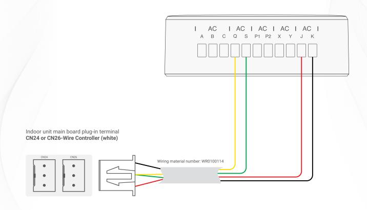
▲ TIS Ducted AC Gateway & Carrier Electric Wiring Guide
