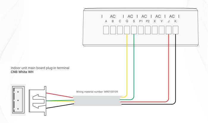
▲ TIS Ducted AC Gateway & Mitsubishi Heavy Industries Multi-Connection **Three-Core Wiring Guide**
