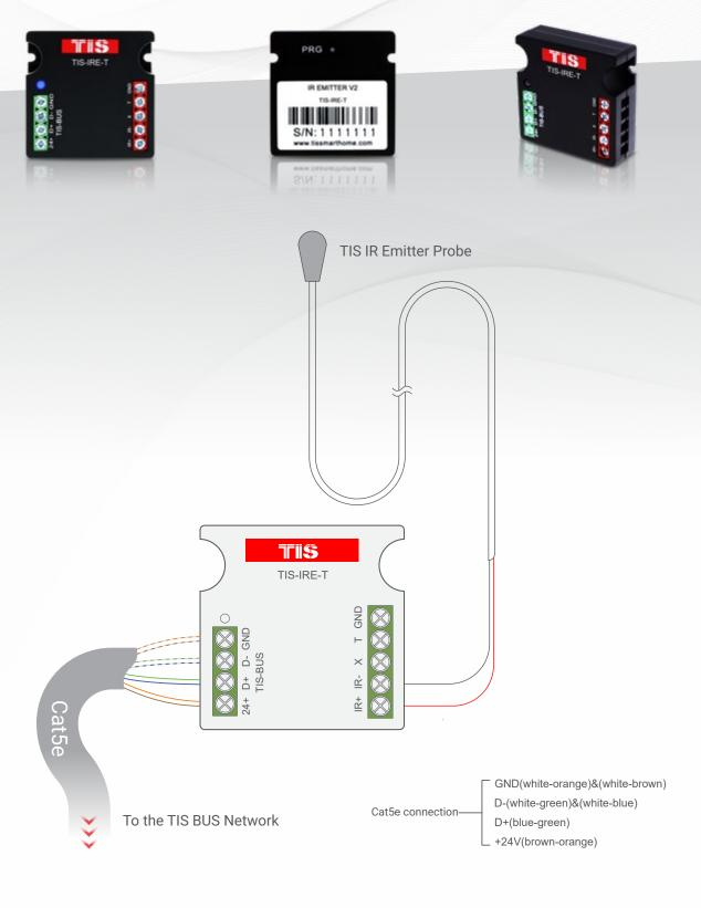
Figure 1: TIS IR Emitter probe Connection Diagram
