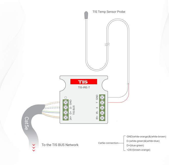
Figure 2: TIS Temperature probe Connection Diagram
