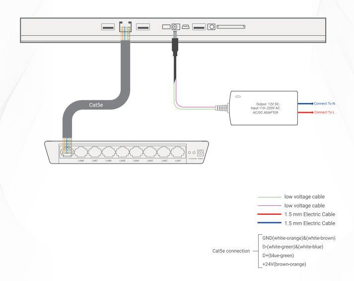
Saturn & network switch & power supply connection diagram (Connect to TIS-BUS network via power switch and Ethernet cable)
