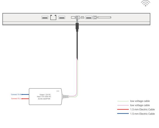
Saturn switch connection with power supply connection diagram (Connect to TIS-BUS network via WiFi)
