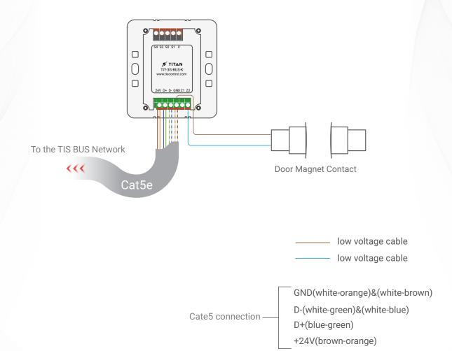
Figure 3: TIT-3G-BUS-K & Magnetic Door Contact Connection Diagram
