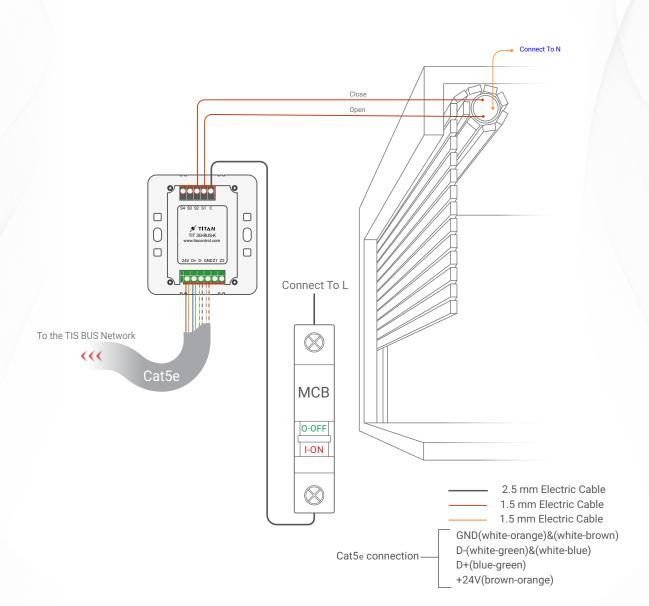
Figure 2: TIT-3G-BUS-K & Motors Connection Diagram
