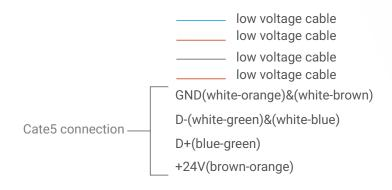
Figure 4: TIT-3G-Bus-K & 3rd Party Sensor Connection Diagram
