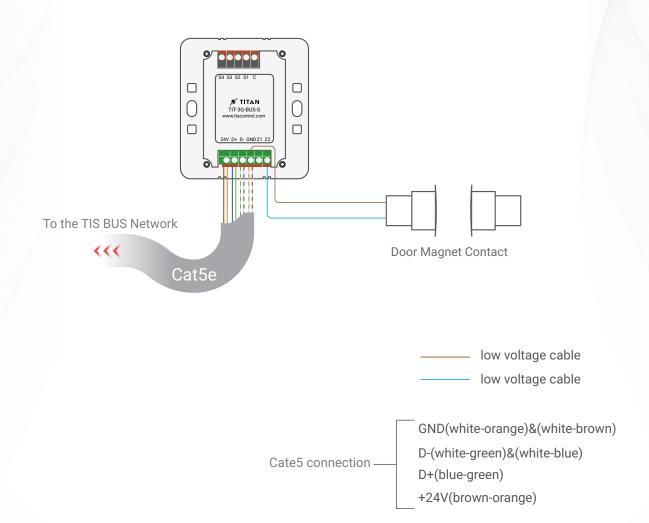
Figure 3: TIT-3G-BUS-S & Magnetic Door Contact Connection Diagram
