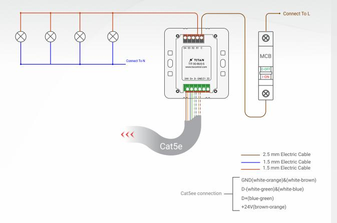
Figure 1: TIT-3G-BUS-S & Lights Connection Diagram
