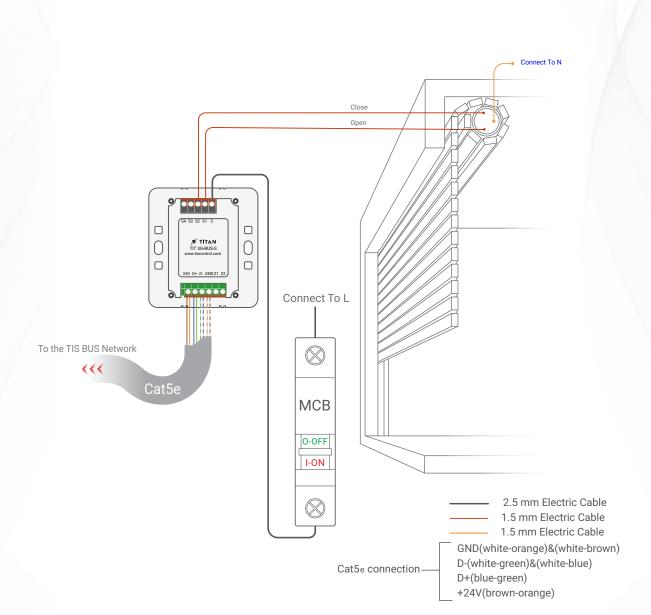
Figure 2: TIT-3G-BUS-S & Motors Connection Diagram
