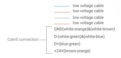
Figure 4: TIT-3G-Bus-S & 3rd Party Sensor Connection Diagram
