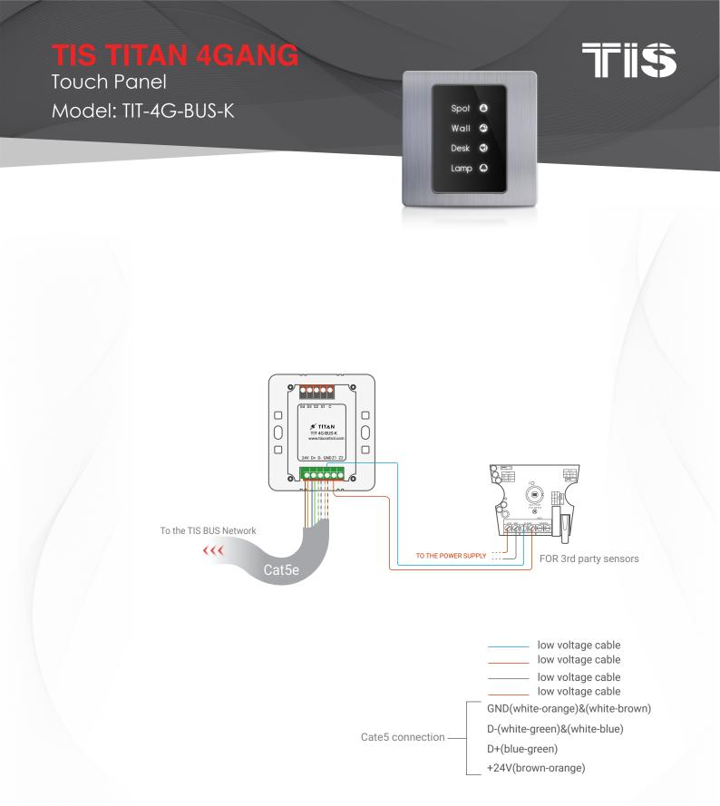
Figure 4: TIT-4G-Bus-K & 3rd Party Sensor Connection Diagram
