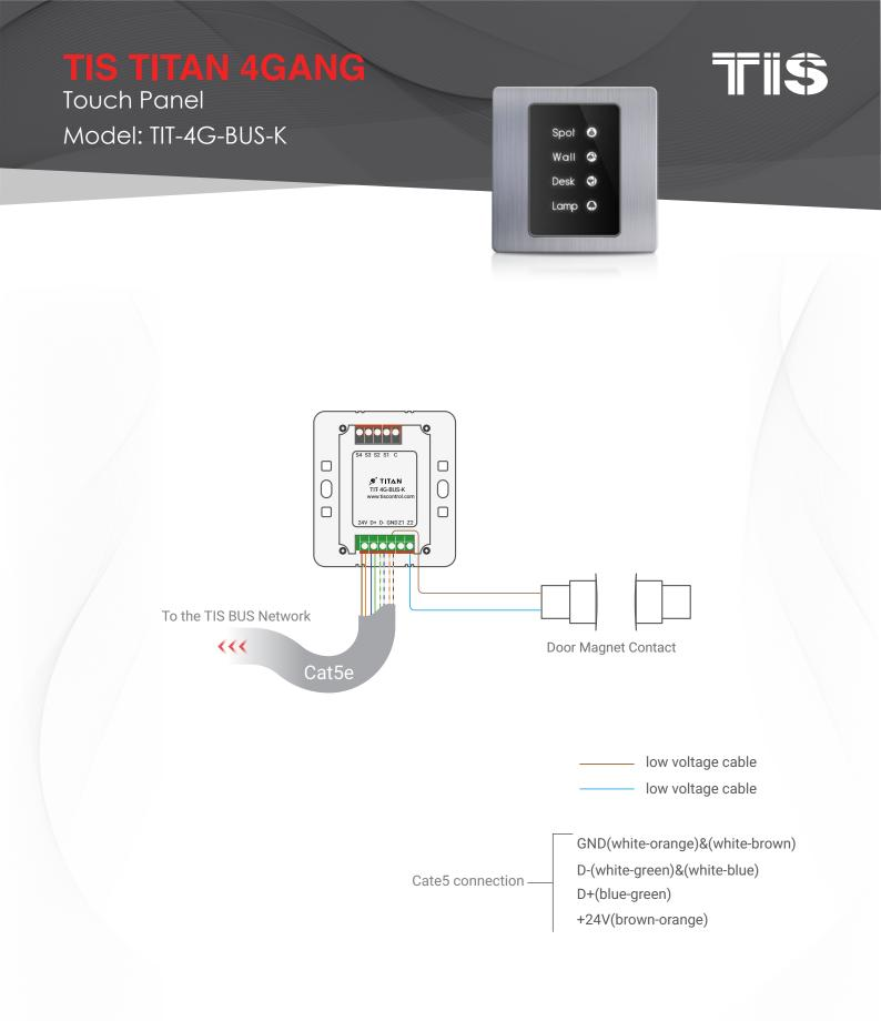
Figure 3: TIT-4G-BUS-K & Magnetic Door Contact Connection Diagram
