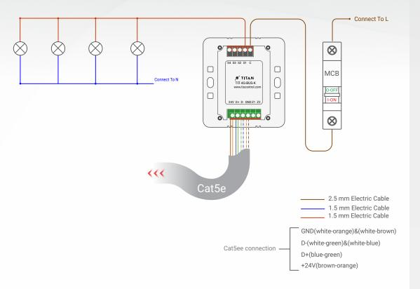
Figure 1: TIT-4G-BUS-K & Lights Connection Diagram
