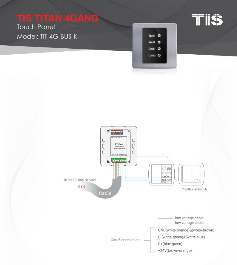
Figure 5: TIT-4G-Bus-K & Traditional Switch Connection Diagram
