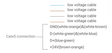
Figure 4: TIT-4G-Bus-S & 3rd Party Sensor Connection Diagram
