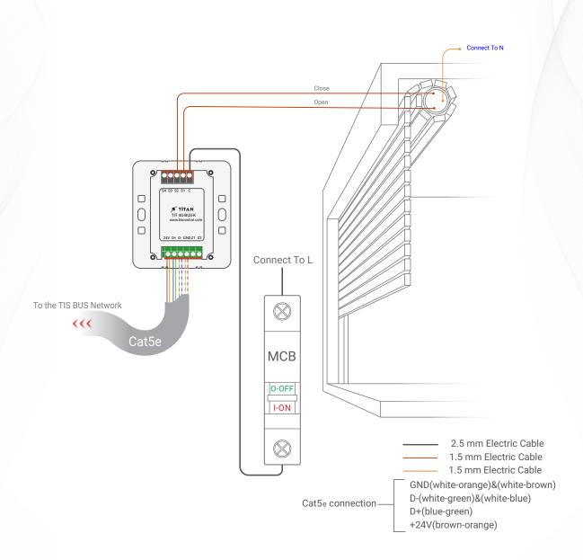
Figure 2: TIT-4G-BUS-S & Motors Connection Diagram
