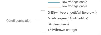
Figure 5: TIT-4G-Bus-S & Traditional Switch Connection Diagram
