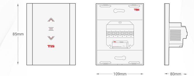
Figure 2: Module's Dimension Diagram
