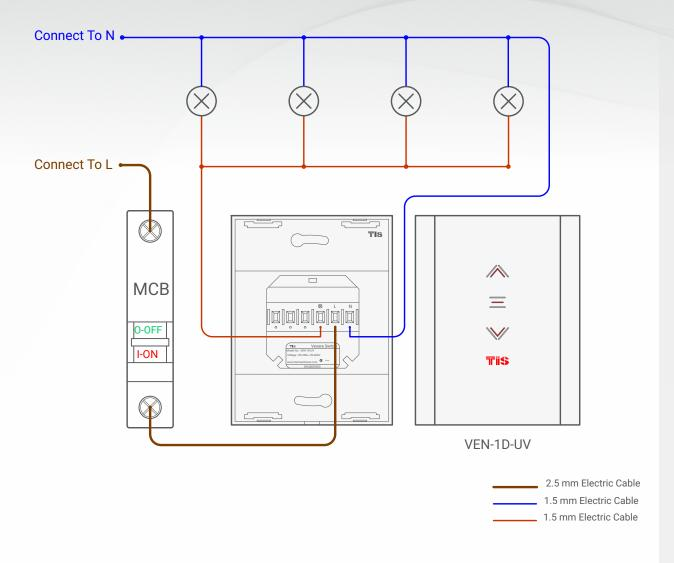
Figure 1: VEN-1D-UV Lights Connection Diagram
