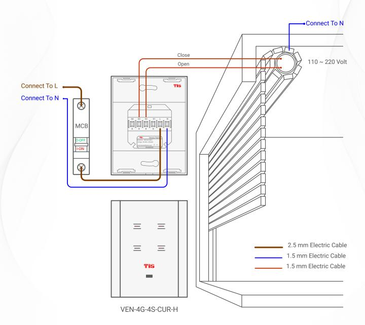
Figure 2: VEN-4G-4S-CUR-H Motors Connection Diagram
