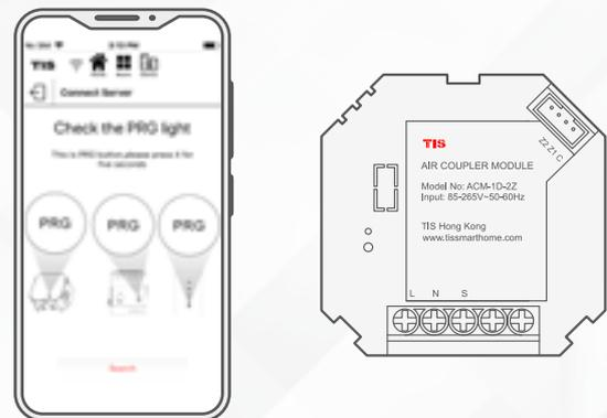
**11** If the module works accurately, then insert the ACM Module into the junction box, and fix it to the wall.
