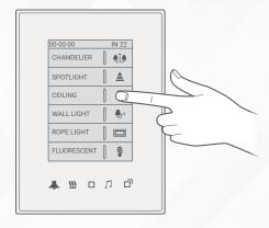
Test by pressing on the wall panel's **3** ON/OFF button. The module relay should respond by turning ON and OFF accordingly.
