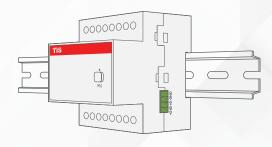
Connect Cat5e TIS network data cable to **3** the TIS-BUS port as per the connection diagram. No need to loop the TIS-bus cable if 2 DIN Rail modules are connected together from the side bus train terminal.
