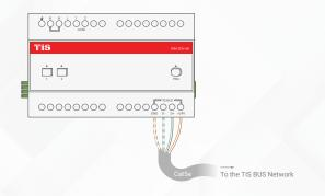
Connect the load (light channel) electrical wires to outputs 1-2. The device is capable of managing up to 10 Amps, and
