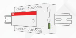
Connect a Cat5e TIS network data cable to the TIS-BUS port as per the connection diagram. No need to loop the TIS-bus cable if 2 DIN Rail modules are connected together from the side bus train terminal.
