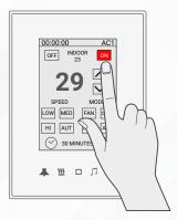
Test your air conditioning by changing **3** the fan speed from low to medium to high. HVAC module should respond accordingly.
