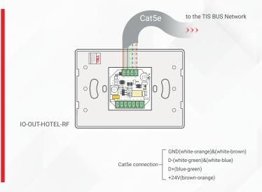
Connect the other connection if needed between wall services switches to the digital inputs of the hotel panel as per the following diagram.
