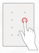
**3** Test the button on the panel by short pressing it for ON/OFF and long pressing it to dim (if channel is dimmable).
