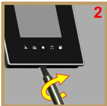
Rotate the screwdriver by 90 degrees.
