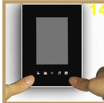
**14** install the upper part make sure the buckles totally inside than push it from down side to be fixed on wall
