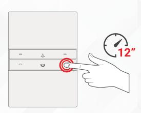
The scene is programmed; you can test it by single press on button 4.
