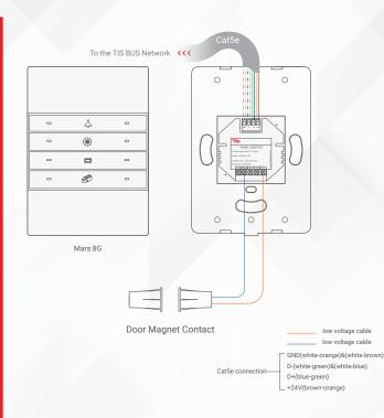
Also, you can connect any 12V operated smoke detector or any 3<sup>rd</sup> party sensor with NC/NO connection to the 12V GND and Z1-Z3 terminals as per the diagram.
