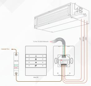
2.5 mm Electric Cable 1.5 mm Electric Cable (GND(white-orange)&(white-blue) D-(white-green)&(white-blue) D+(blue-green) 24+V(brown-orange)
