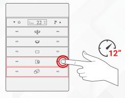
The scene is programmed on the pressed button; you can test it with a single press.
