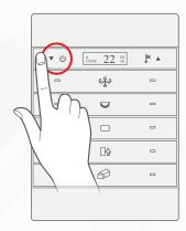
3 D Test your air conditioning by changing the fan speed from low to medium to high. Your relay should respond accordingly.
