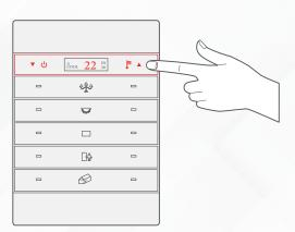
Long press any button from 7-9 for 16 **3** seconds until its LED blinks BLUE.
