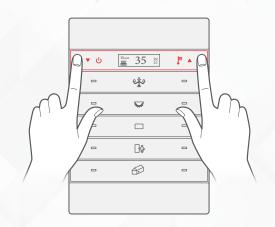
3 D Test your floor heating by changing the temperature, relay should respond accordingly.
