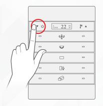
**3** Test your air conditioning by changing the mood, Heat/Cool, and fan speed from low to medium to high. HVAC module should respond accordingly.
