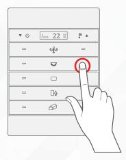
3 D Test the button on the panel by short pressing it for ON/OFF and long pressing it to dim (if channel is dimmable).
