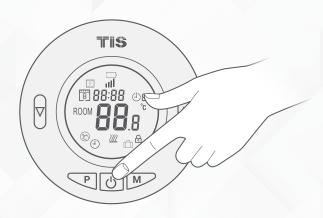
Long press the M button on the TRV for 6 seconds. The graph on the TRV's LCD will change.
