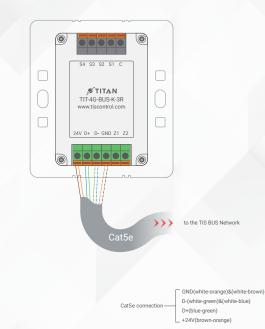
4 ➤ You can connect 2 digital inputs to any switch or window magnet. Connect the digital input wires to GND, Z1, and Z2 terminals, as is shown in the diagram.
