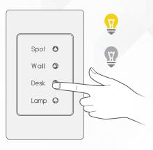
Test the feature by tapping the power button for lights ON/OFF or holding it to dim the light (if the channel is dimmable).
