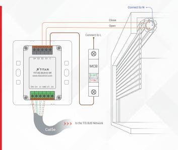
2.5 mm Electric Cable 1.5 mm Electric Cable 1.5 mm Electric Cable GND(white-orange)&(white-brown) D-(white-green)&(white-blue) D+(blue-green) +24V(brown-orange)
