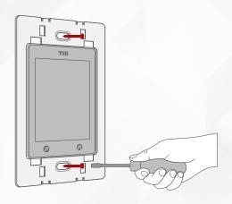
Put the plastic, metal, or glass cover on the main panel and push to fix it in the place.
