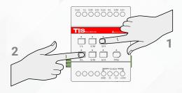
Wait for few seconds until the PRG LED **3** stops blinking.
