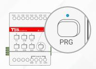
Test by turning the first button ON and 4>> then the second button. Both buttons should not turn ON together. If you see that the first button is turning the other button off, that means that your buttons are successfully combined as shutter/ curtain mode.
