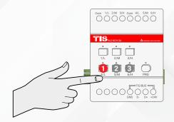
To program the FCU to any wall thermostat panel, press and hold the first Channel L (LOW) button for 6 seconds. The LED indicator of the pressed button will start blinking,
