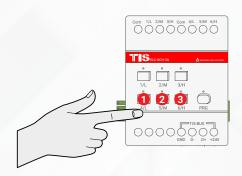
Wait for a few seconds until the PRG LED stops blinking.
