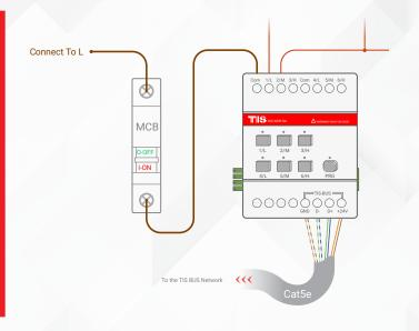
Turn on the power source, and then test the loads by short pressing on the device's local override buttons 1-6.
